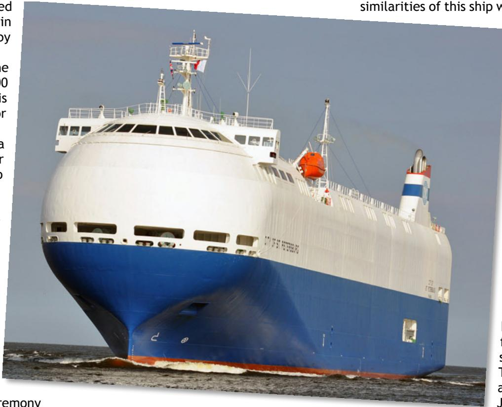
Association (JSEA), was subject to press-bending, giving a relatively distortion-free shape. In making the award, JSNA said that although streamlined hulls had previously been designed in conceptual ships, "its first realisation [in this ship] has been highly appreciated." In addition to the forebody, the offset funnel is streamlined and the upper
